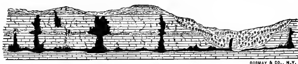
FIG. 53. — Relations of caverns at two levels to sink holes above, springs on a valley side, and a natural bridge. (After Shaler.)
